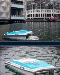
Powered by batteries, the WasteShark boasts an impressive range of up to five kilometres on a single charge, equivalent to eight to 10 hours of continuous cleaning. Every day, this environmental sentinel manages to extract approximately 500 kilograms of waste, equivalent to around 21,000 bottles.
